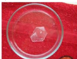
Fig.1. (a) Grown crystal of KAP doped with NaCl ;( b) Grown crystal of KAP doped with LiCl
