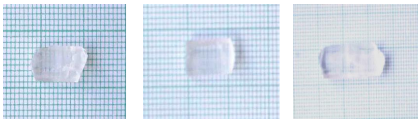
Fig 2. Photographs of the as grown (a) pure LAM, (b) \text{La}^{3+} -LAM and \text{Nd}^{3+} -LAM crystals
