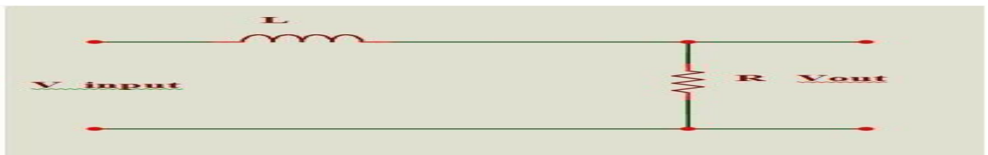
Fig. 4 Circuit diagram of passive Low Pass filter
