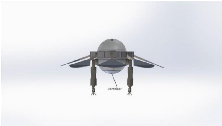
Figure 2: Front view of the octopus-like AUV.
