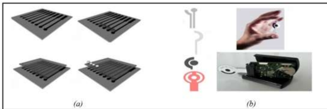
Figure 2: (a) Screen-printed electrodes for pH detection [7] ; (b) Portable equipment for ammonium ion detection [9]
