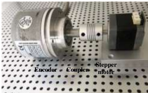
Figure 15: The installation for measuring the rotational deviation of motor with 16-bits high-precision optical encoder.
